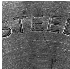
BF Incident lighting
