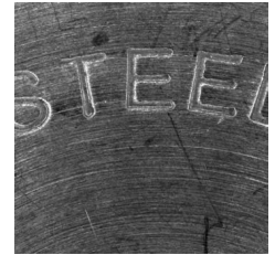
BF + DF Incident and grazing lighting
